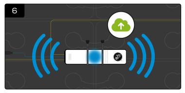
The radio is now enabled, and the blue LED remains illuminated until all data has been transmitted to eGO!cloudlink.
