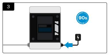
Connect the eGO!cloudlink with power connection. And wait for 90 seconds.
