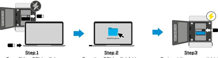
Turn off the eGO!cloudlink. Eject the memory stick and insert it into a PC.
