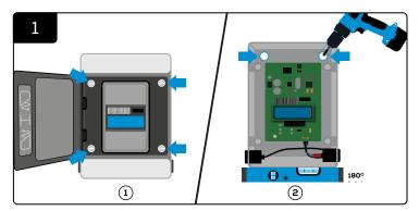
Open and unscrew the grey cover. Mount the control box to the wall using four screws/anchors and a level. Make sure it is firmly attached to the wall. Rescrew the cover.
