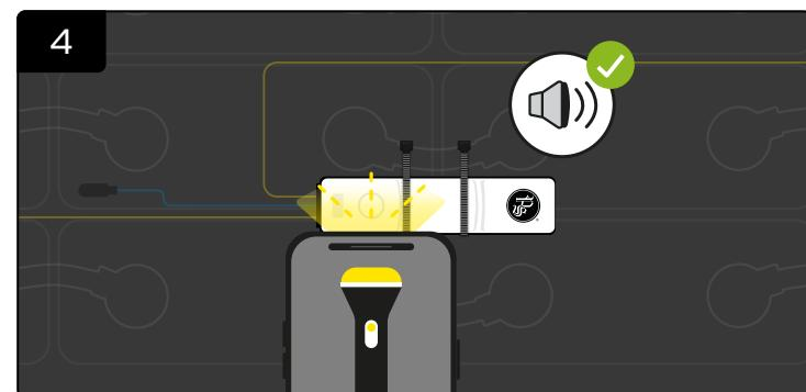
Take a bright flash light (\*A mobile phone flash light will be adequate) and place directly on **top of the white circle on eGO! monitor** until you hear a beep along with blue LED.
