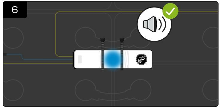
At this point quickly remove the flash light and you should hear a second beep.
