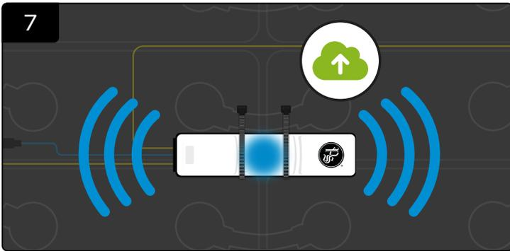
The radio is now enabled, and the blue LED remains illuminated until all data has been transmitted.
