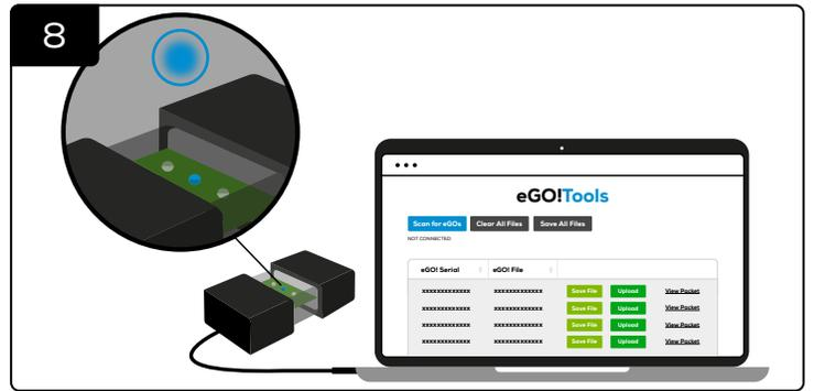
If data uploads successfully to eGO!Tools, blue LED will also illuminate on eGO!Receiver. eGO! data packets will appear in the list, along with the voltage logs.
