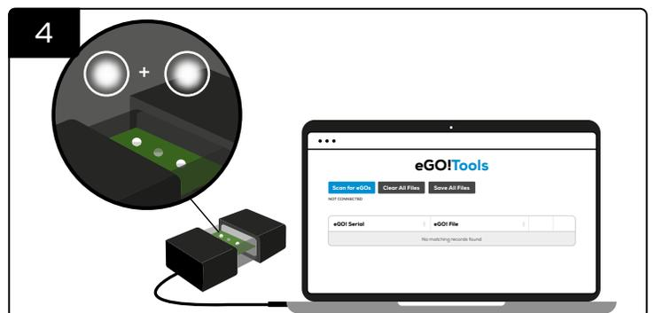
If the flashing white LED becomes solid (2 solid white LEDs), the eGO!Receiver is successfully connected to the eGOs serial port.
