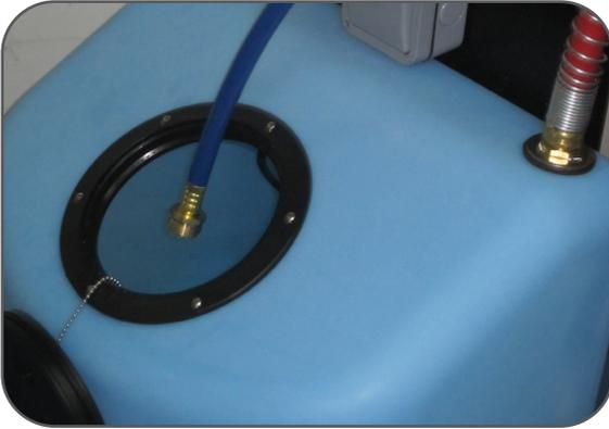
Remove packing material from the tank. Fill the tank to the desired level with deionized water.
