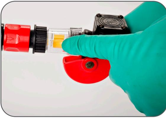
Watch the spinner mounted on the Instant Valve Pro. When it stops spinning, the filling is completed (about 15 seconds, usually). Note: The spinner may not come to a complete stop, especially in larger systems. The battery is filled when the spinner slows enough to clearly see the inner blades/vanes.
