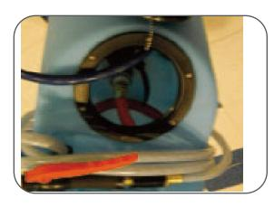
Remove packing material from the tank. Fill the tank to the desired level with deionized water.
