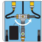
Rotate the Selector Valve to choose the next cartridge.
