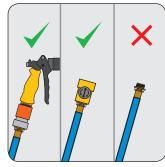
Attach either a **Watering** *Gun* or Flow Restrictor to the free end of the blue Output Hose.
