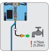
Connect the free end of the black inlet hose to the water supply (fittings supplied).
