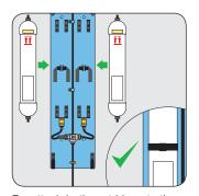
Re-attach both cartridges to the mounting plate using the straps. Ensure arrows are pointing up.
