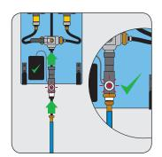
Attach the battery case as shown followed by the Purity Light and blue Output Hose to the selector valve.
