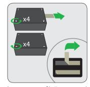
Loosen screws of battery case and pull out tape to activate. Re-tighten screws and remove backing tape from the velcro strips.
