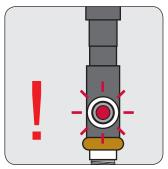
If the Purity Light flashes red then the cartridge needs replacing.
