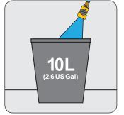
Pass 10 Litres (2.6 US Gallons) of water through the system into a bucket.
