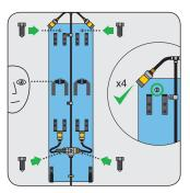
Securely attach the mounting plate vertically to the wall with the strap fitting at eye-level.
