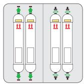
Remove the red caps from both cartridges and thread on the 2 male quick-connect fittings.
