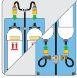
Re-attach the 4 black hose connectors to the top and bottom of the cartridge.
