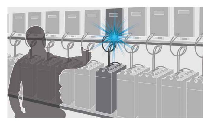
iBOS Lite manages up to 50 chargers for each battery type and uses easy-tosee pick lights to provide clear direction on which charged battery to select.
