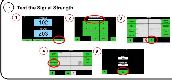
If "Received" is not greater than 95, the antenna may need to be relocated to improve the signal strength.
