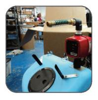
Ensure that when the HydroTronic Control Unit is secured that the hose is facing the front of the tank.
