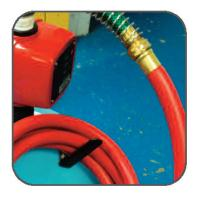
Attach the heavy duty hose to the strain relief hose.
