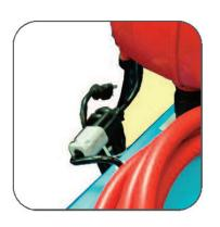
Plug the cord on top of the tank into the HydroTronic and plug the HydroTronic into the 110-120 VAC outlet on the battery changer.
