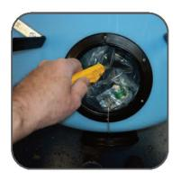
Open fill cap and using a utility knife, puncture the packing material around the pump.
