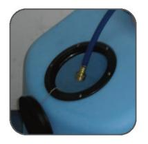
Remove tank lid and fill tank with deionized water.
