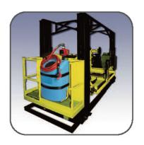
Secure tank assembly to the back of the battery changer. Installation of a uni-strut welded to the back of the operator's platform may be necessary
