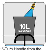
"OFF" position to the "LEFT" position to open the water flow to the cartridge. Pass 10 Liters (2.6 US Gallons) of water through the system into a bucket.
