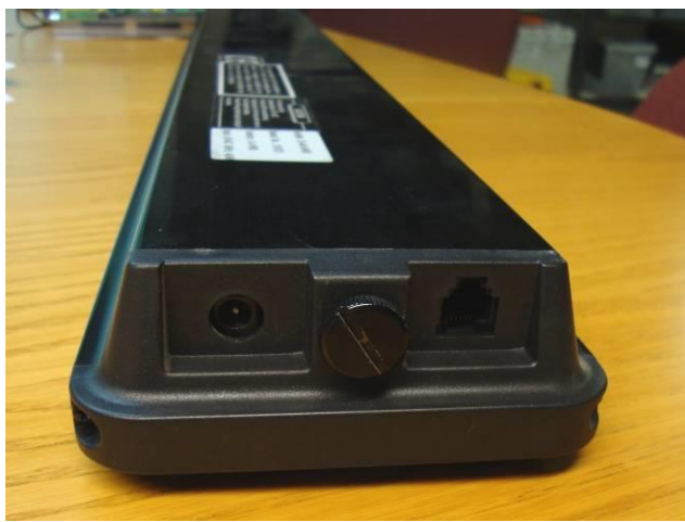
Type A Scrolling Displays: Are labeled on the back for use with “Use with 9 VAC”. Type A signs also use a telephone cable (RJ11) for a data connection.
