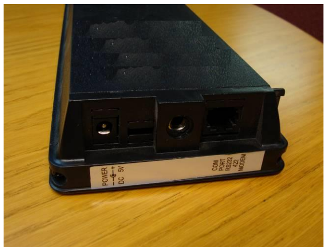
Type B Scrolling Displays: Are labeled on the side with “Use with 5 VDC”. Type B signs also use a Cat 5 cable for data connection.
