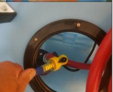
Once the tank is full, prime the pump. Aim the Instant Valve into the tank, squeeze the valve and hold it open. Press and hold the start button until the unit displays "Priming" Hold the start button and the IVP simultaneously for five seconds, release the start button and then release the IVP.
