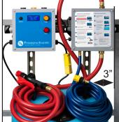
Install the connector hose from the end of the brass fitting assembly to the top of the Pressure Control Module as shown.
