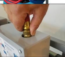
Install the hose and IVP without spinner assembly to the bottom right of the gray box. The IVP with the spinner must not be used with this system. If the IVP with the spinner is to be kept as a spare, the spinner must be covered with tape.
