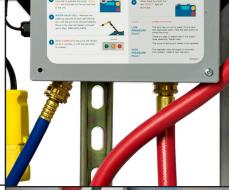
Plug the pump cord from the tank into the yellow receptacle on the pump controller. Plug the unit into the extractor to turn on the system. Secure the excess wire to the frame with provided cable ties.
