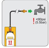
Connect the free end of the black inlet hose to the water supply.
