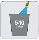
Pass19 - 38 Litres (5 - 10 US Gallons) of water through the system into a bucket.
