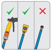
Attach either the **Watering** *Gun* or Flow Restrictor to the free end of the blue hose
