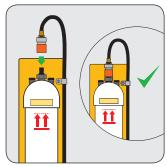
Connect the fixed end of the black inlet hose to the cartridge.
