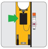
Attach the battery case firmly to the velcro strips on the backplate.
