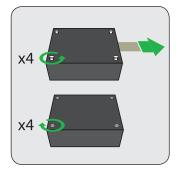
Loosen 4 screws of battery case and pull out tape to activate. Re-tighten screws.
