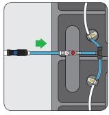
The water stops automatically. Disconnect the water supply.
