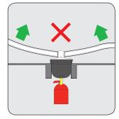
Do not try to remove the AFS by pulling on the tubing.
