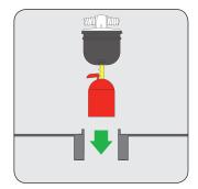
Place an AFS into the vent hole of each battery cell and press firmly into place.
