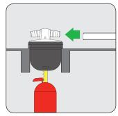
Fully push the free end of the tubing on to the first AFS and push until it stops.
