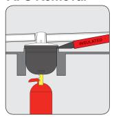
Remove by inserting an insulated screwdriver (or similar) under the lip of the AFS.
