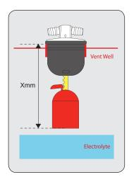
Check manufacturers guidelines for fill heights. If the there are no guidelines available then always use the longest setting possible, ensuring there is a 5mm gap from the top of the separators to the underneath of the float in the extended position.
