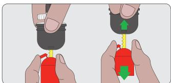
Pull the pin back and then move the float to the required position.
