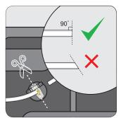
Cut the tubing square at this point using a tube cutter or scissors ensuring end of tubing is not crushed.
