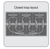
With the remaining tubing securely connect all of the AFS together in the same way.
